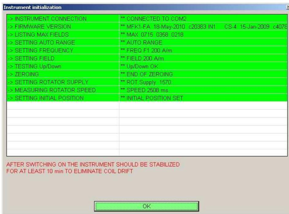
**Figure 5:** *Instrument initialization window.*
