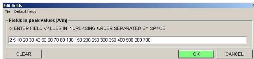
Figure 16: A window for editing the sequence of fields intensities.
