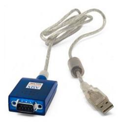
Another brand can be used, but the converter MUST be equipped with **FTDI** chip which provide full USB to RS232 conversion. After installing drivers for the converter it is necessary to assign COM port number of such converter to 1 or 2 with respect to the value written in the configuration file.
