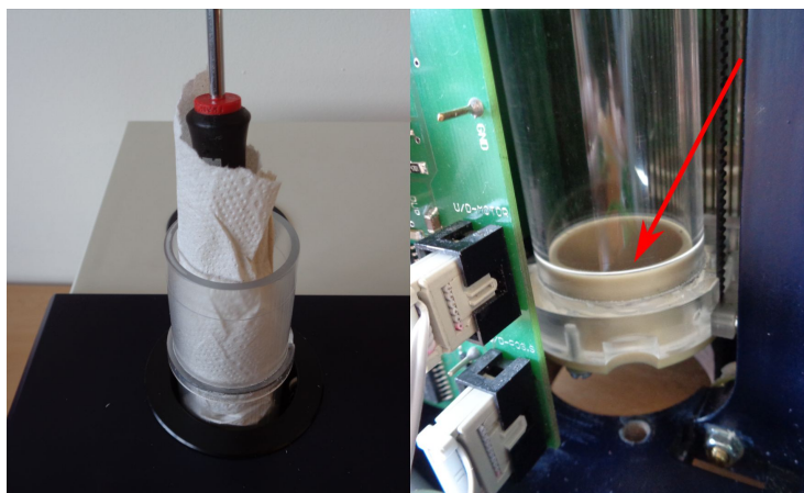
Figure 7: Cleaning of tube
